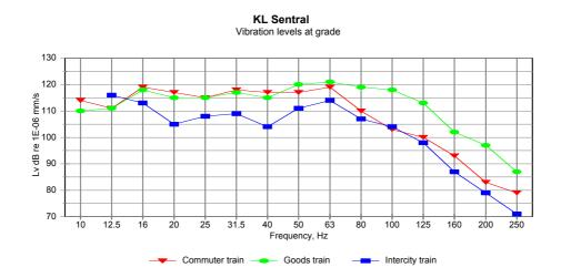
The project performance specification sets the criteria for ground-borne vibration within the station as less than the curve specified in ANSI Standard S3.29/1983 (vertical axis). For critical areas such as the VIP lounge, the maximum acceptable curve was 1.4 (0.14mm/s in the range 100-250 Hz).
