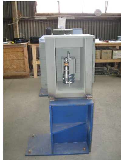
Figure 12. End view of variable frequency TMD showing dashpot and spring during commissioning.
