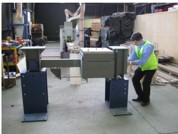
Figure 11. Side view of variable frequency TMD, during factory testing.
