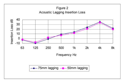
Two alternative lagging options were developed, one nominally 50m thick and with a 5kg/m² wrap and the other nominally 75mm thick with a 6kg/m² wrap. The densities of the 50mm Rockwool insulation were 65kg/m³ and the 75mm Rockwool lining was 80kg/m³. The insertion loss of these lagging alternatives are given in Figure 2.
